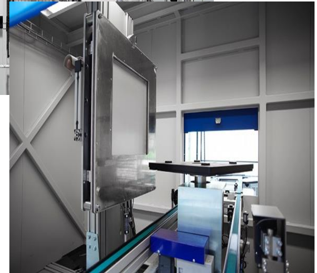
HeiDetect XS CT: Blick in die Inline CT Maschine
